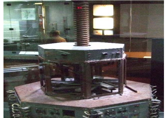
This strange device was used to test how various materials and electronic components would react to a nuclear blast.
