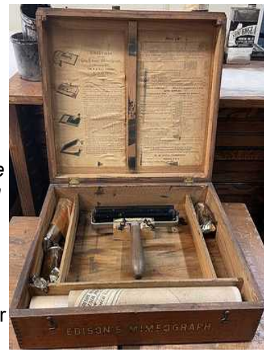
The earliest Edison Mimeograph, produced by AB Dick, a flatbed device.
