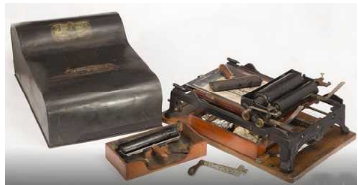
An Edison Automatic Mimeograph No 51, 1898, a middle stage in the development. The flatbed has fixed rollers, probably driven by the crank laying below.
