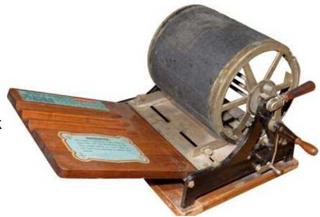
A very basic 1909 mimeo., with recently invented rotating drum. On the blue paper attached you can barely make out: Gestetner.
