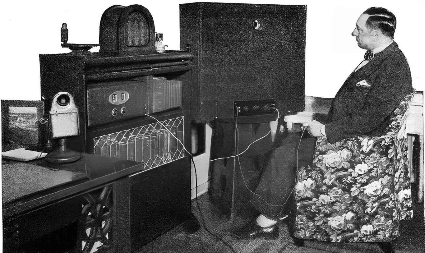
H. Gernsback, Editor of RADIO NEWS, receiving the television broadcasts from WRNY home in New York City, with the simple apparatus described in this article. For purp test, the neon tube and loud speaker were connected in series temporarily, with operation simultaneously.
