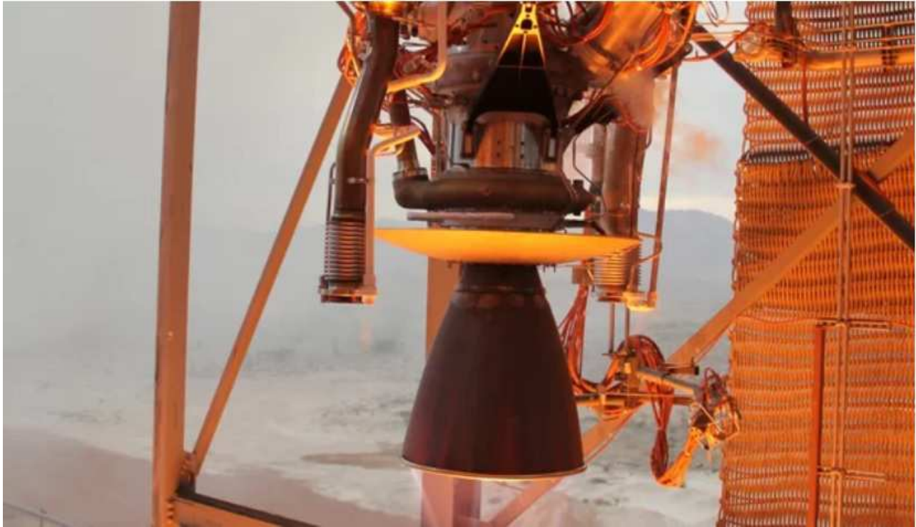
Blue Origin's BE-3 throttles during acceptance testing. Credit: Blue Origin
