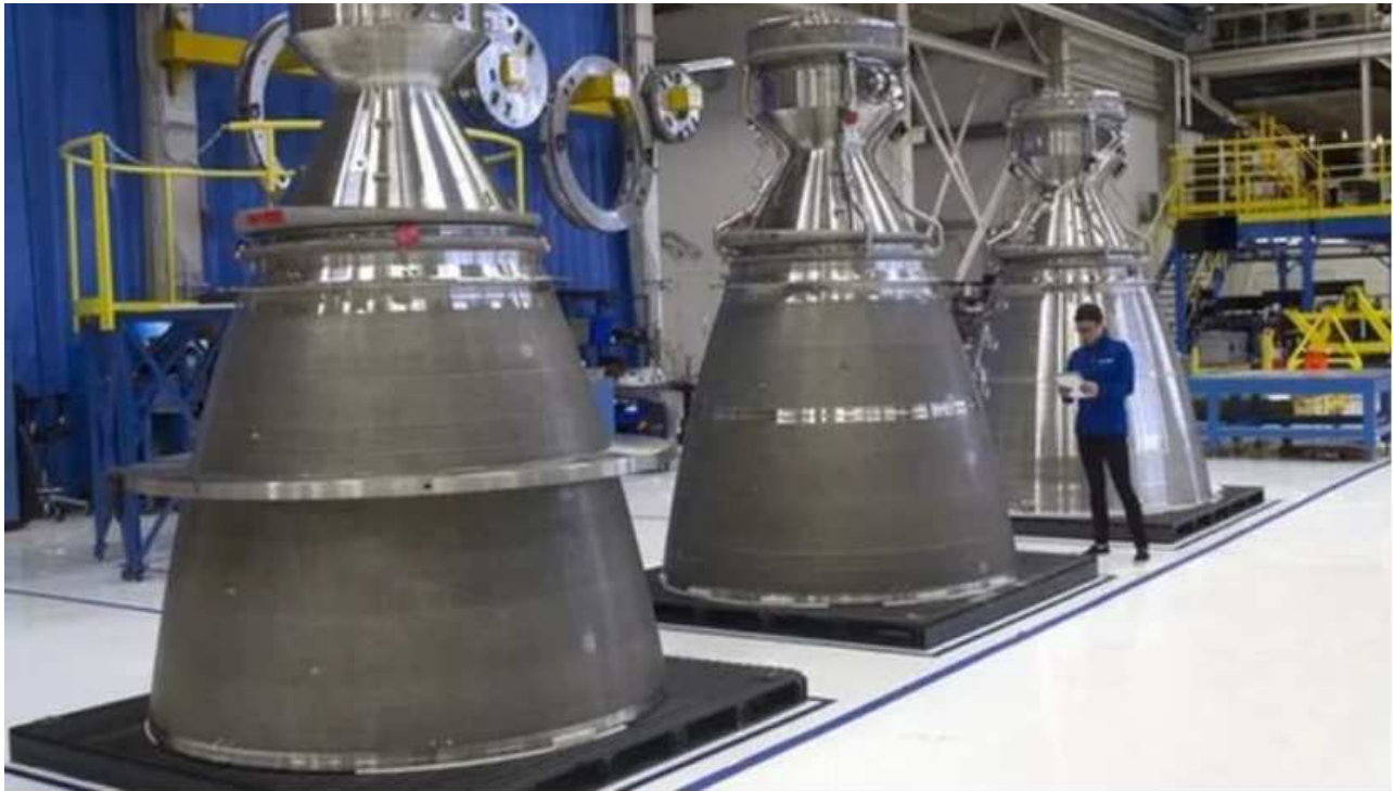
A group of BE-4 engines being assembled at Blue Origin's Kent, Washington, facility. Credit: Blue Origin
