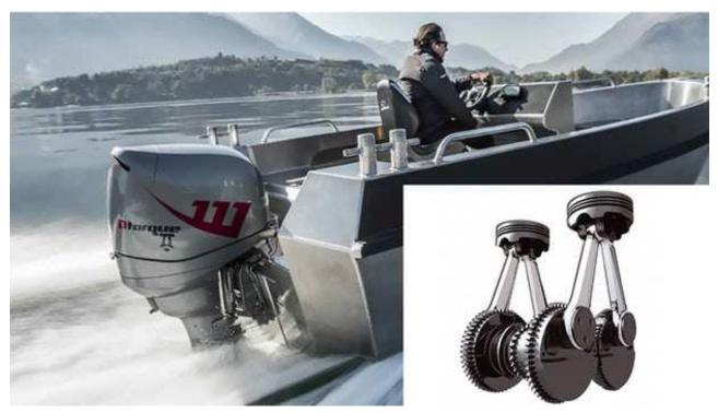
Compared to petrol outboards, the Yanmar is lighter, smoother, more compact, has double the engine life, and offers much better fuel consumption and running costs. It produces less toxic emissions, has more torque much lower in the rev range and that's before you consider the safety and ready availability of diesel fuel.(Credit: Yanmar/Neander-Motor)
