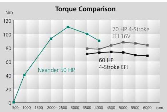
The Dtorque 111 is named for its remarkable low rpm torque, with 111 Nm on offer at 2,500 rpm. That's the type of grunt that will immediately fling a medium-sized boat onto the plane, offering a far different experience than a high revving traditional four-stroke.
