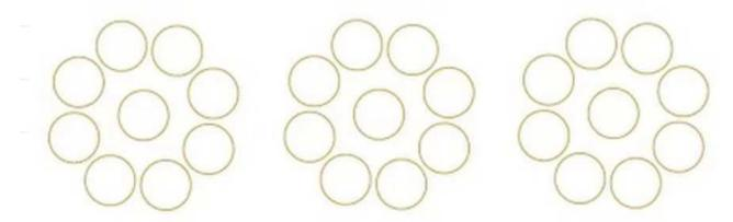
The 27 Merlin engines that power the Falcon Heavy's three cores are arranged in an "Octaweb" configuration. Credit: SpaceX
