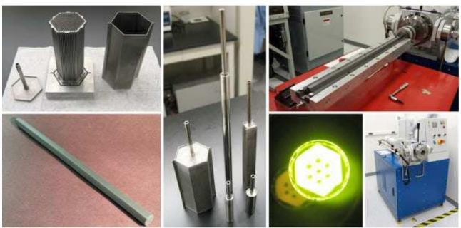
Advances in materials technology could lead to the production of LEU NTP fuel elements (Credit: NASA)
