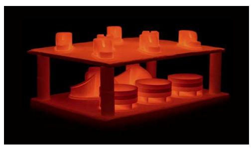
Sintering **Multiple** Parts -Desktop Metal's Studio System includes a fully-automated, office-friendly sinterina furnace with fast cycle times and a peak temperature 1400°C, allowing for the sintering of a wide variety of materials. (Credit: **Desktop Metal)**
