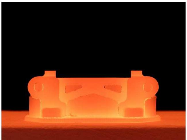
Depending on the nature of the part, it might be necessary to do some post-print surface finishing like sanding or bead blasting to smooth out the layered surfaces, but effectively you're left with a prototype part, produced quickly, in the production material and ready for testing. And parts are around 99.8 percent dense, which is huge. They're very mechanically tough.
