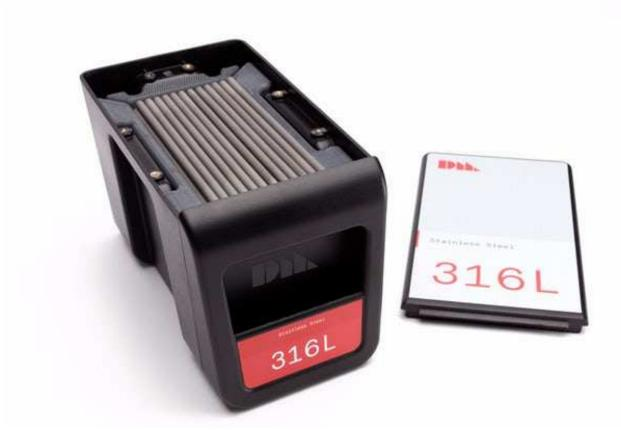
The Studio printer runs around and prints parts into layers of bound metal. The parts then go into a de-binding bath that removes a good portion of the binding polymer, and then the parts go into a sintering furnace.
