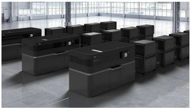
The rest of the process – de-binding and sintering – looks much the same as the Studio system. Print resolution is as fine as 50 microns, roughly the width of a human hair. And while no final pricing has been given yet on the full system, each printer will retail for around US\$360,000.
