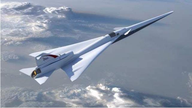
Illustration of NASA's planned Low Boom Flight Demonstration aircraft as outlined during the project's Preliminary Design Review (Credit: NASA/Lockheed Matin)
